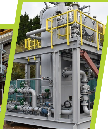
INDUCTED GAS FLOTATION
