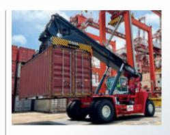
At SAGT, DIMO was involved in commissioning the Kalmar Essential Reachstacker DRU45, which is capable of handling ISO 20'/40' laden high cube containers in a 5 high and three deep stacks. The machine's lifting capacity beneath the spreader is 45 tonnes and it is equipped with the Kalmar adjustable 20' - 40' spreader with a side shift of =/-800mm.
