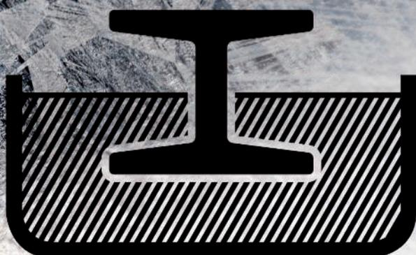
“Batch galvanisation” is mainly used for galvanising prefabricated steel parts.
